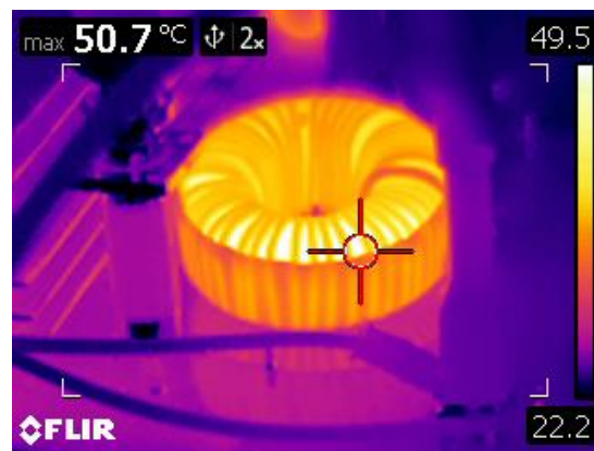
Figure 22. Thermal Scan of Inductor
