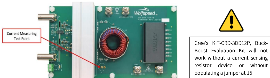
Figure 16. Current Measuring Test Point on Cree's KIT-CRD-3DD12P, Buck-Boost Evaluation Kit
