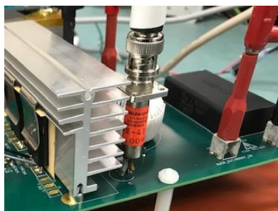
Figure 15. Cree's KIT-CRD-3DD12P, Buck-Boost Evaluation Kit with Current Viewing Resistor Installed
