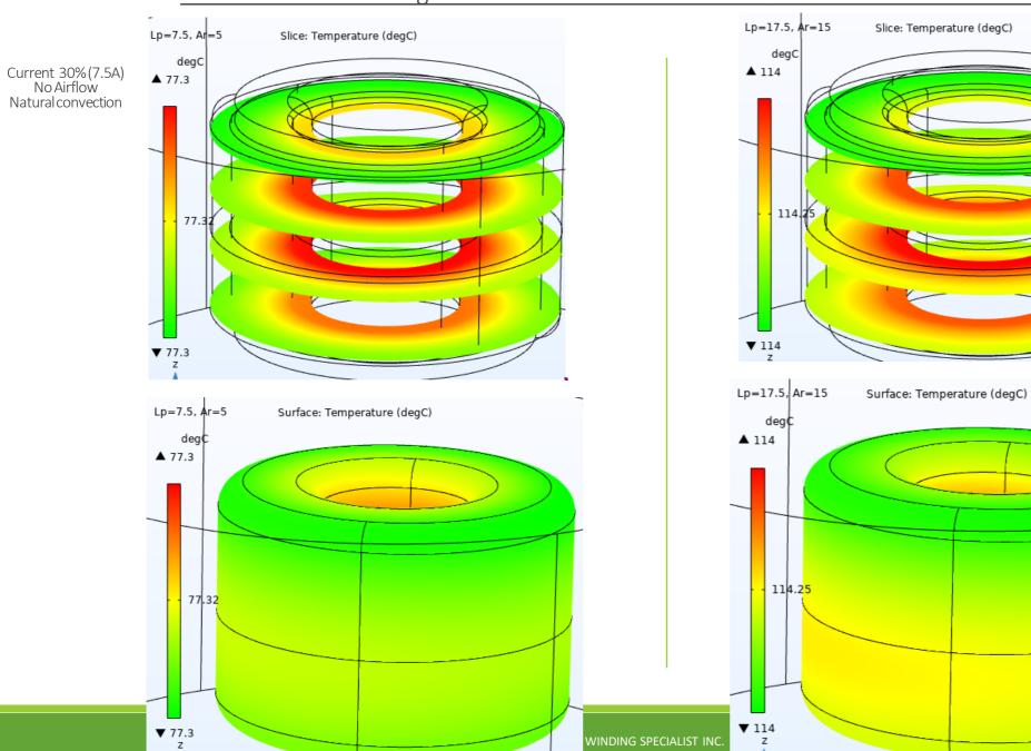
Current 70% (17.5A)  $15 \text{ W/ (m}^2\text{K) or } 3 \text{ m/s}$  air flow.
