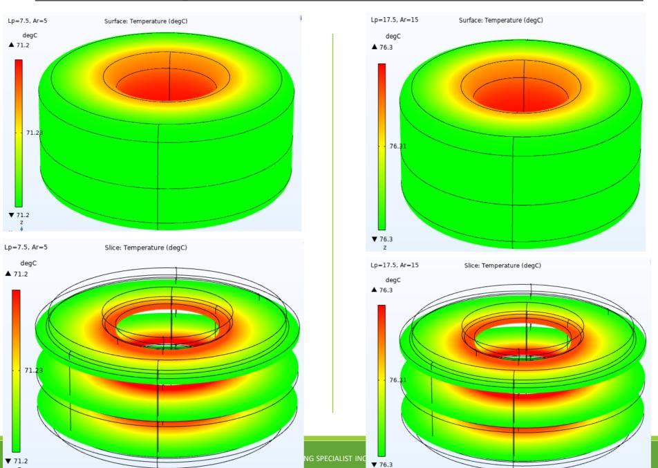
Current 70% (17.5A)  $15 \text{ W/ (m}^2\text{K) or } 3 \text{ m/s}$  air flow.
