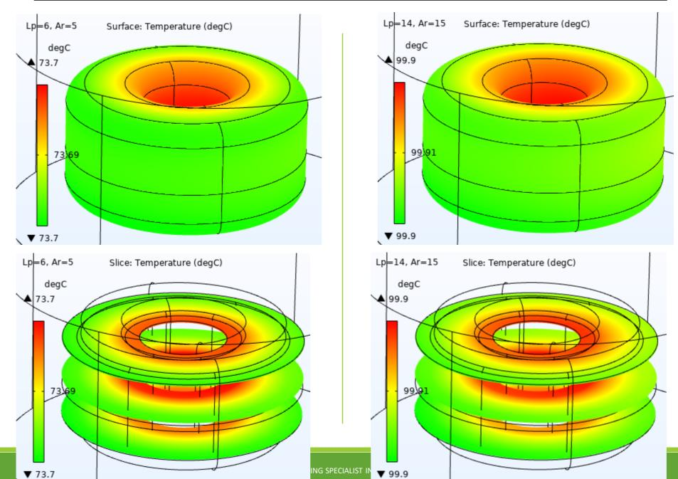
Current 70% (14A)  $15 \text{ W/ (m}^2\text{K) or } 3 \text{ m/s}$  air flow.
