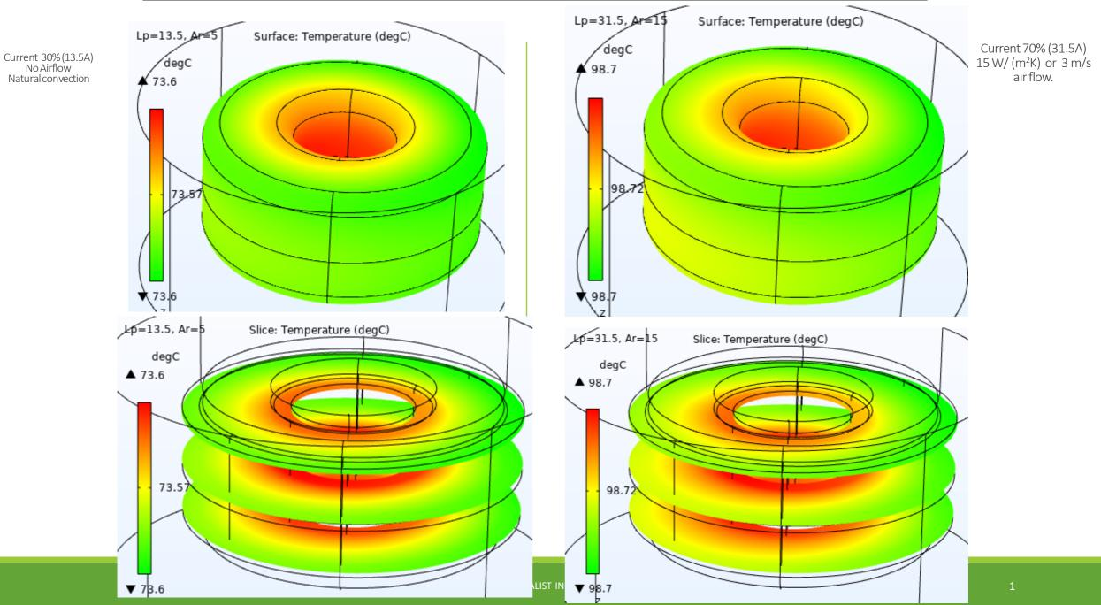
Thermal and Electromagnetics simulation – Part # HF467-260M-45AH – Current rated 45A @ 1kHz
