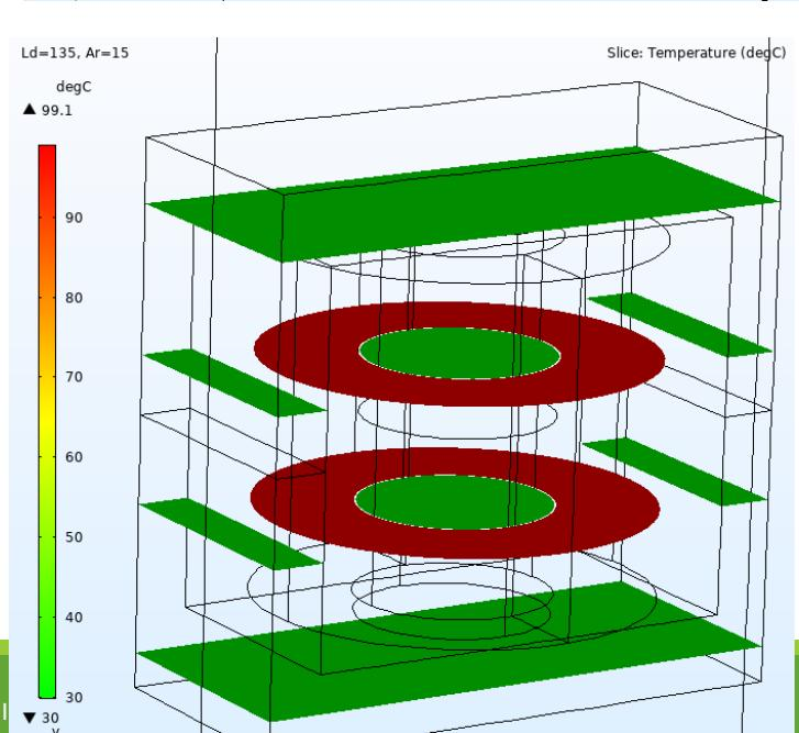
Thermal and Electromagnetics simulation – Part # E70340-010 – Current rated 180A @ 10kHz
