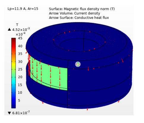
Lp=11.9 A, Ar=15 Arrow Volume: Magnetic flux density Volume: log(mf.normJ)
