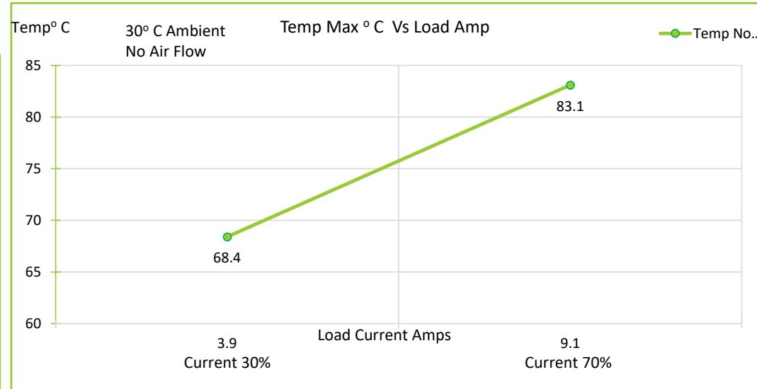
Thermal and Electromagnetics simulation – Part# SN270-330M-13.0AH– Current rated 13A @ 1kHz
