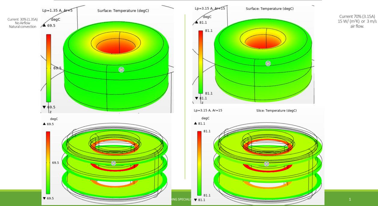
Thermal and Electromagnetics simulation – Part #SN270-471M-4.5AH– Current rated 4.5A @ 1kHz
